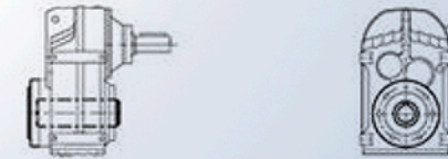
Serie EF.S (entrada y salida de eje sin motor) EF.S Series (shaft input and output without motor)
